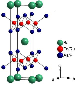
FIG. 1: (Color online). Crystal structure of  $\text{BaFe}_2\text{As}_2$ . There are two ways for isovalent substitution in the  $\text{Fe}_2\text{As}_2$  slabs, substituting As with P, or Fe with Ru. Both substitutions can induce superconductivity, and result in similar phase diagrams.
