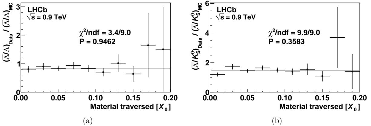
Figure 4: The double ratios (a)  $(\bar{N}/A)_{\text{Data}}/(\bar{N}/A)_{\text{MC}}$  and (b)  $(\bar{N}/K_S^0)_{\text{Data}}/(\bar{N}/K_S^0)_{\text{MC}}$  are shown as a function of the material traversed, in units of radiation length. Flat line fits, shown together with their respective  $\chi^2$  probabilities, give no evidence of a bias.
