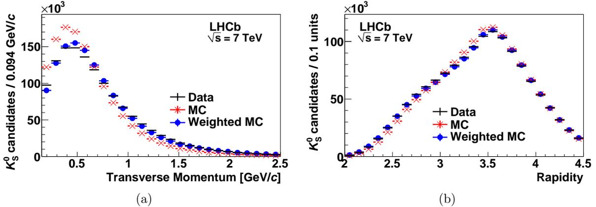
Figure 3: (a) Transverse momentum and (b) rapidity distributions for  $K_S^0$  in data and Monte Carlo simulation at  $\sqrt{s} = 7$  TeV. The difference between data and Monte Carlo is reduced by weighting the simulated candidates.
