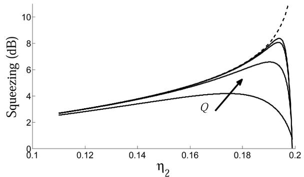
FIG. 2. Squeezing generated by dissipation in a single-mode microwave cavity:  $\omega_0 = 3.5$ ,  $\epsilon = 10$ ,  $\gamma_q = 0.2$ ,  $g = 1$  GHz, and  $\eta_1 = 0.2$ . We have used Eq. (10) and the definition of squeezing in the main text. Continuous lines correspond to  $Q = \omega_0/\kappa = 10^{5,6,7,8}$ , and the dotted line is the ideal squeezed vacuum generated by  $\mathcal{L}_{\text{sq}}^{[s]}$ .
