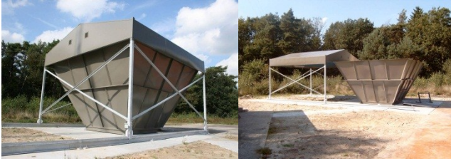
Fig. 1 a) THACO, a) with roof in the 'hot load' position and b) with roof removed, for the 'cold load' measurement
