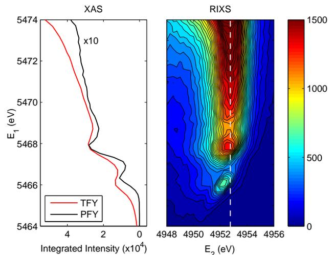
FIG. 3. (Color online) (a) V K pre-edge X-ray absorption spectra in a  $(\text{V}_{0.989}\text{Cr}_{0.011})_2\text{O}_3$  single crystal measured at room conditions in the partial (PFY) and total (TFY) fluorescence modes; (b) RIXS surface as a function of incident ( $E_1$ ) and emitted ( $E_2$ ) photon energy in the vicinity of the pre-edge region.
