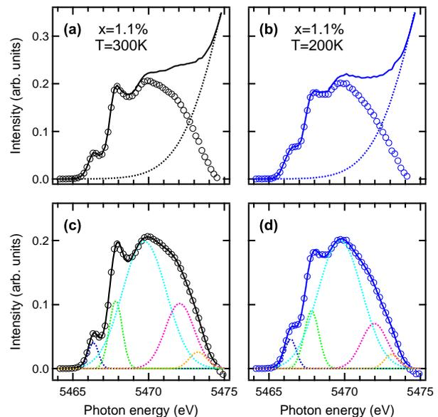
FIG. 9. (Color online) Illustration of the pre-edge fitting procedure for the data obtained on the  $(V_{0.989}Cr_{0.011})_2O_3$  sample across the temperature induced MIT: after subtraction of the dipolar tails (dotted lines, top panel), the remained features (circles) are fitted using five gaussian functions (dotted lines, bottom panel). The maxima of the first two gaussians corresponding to the peaks A and B are used to display the  $I(A)/I(B)$  evolution in Figure 10(d-f).
