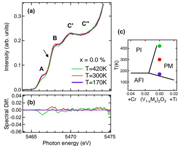
FIG. 6. (Color online) V-K pre-edge X-ray absorption spectra for a  $V_2O_3$  (PM) powder sample as a function of temperature in PFY mode ( $T=170K, 300K, 420K$ ); (b) spectral differences, with respect to the low temperature spectra; (c) corresponding points in the phase diagram.
