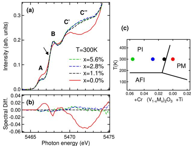
FIG. 5. (Color online) V-K pre-edge X-ray absorption spectra for a  $(V_{1-x}Cr_x)_2O_3$  powder sample at room conditions as a function of doping ( $x = 0, 0.011, 0.028, 0.056$ ) in PFY mode; (b) spectral differences, with respect to the  $x = 0.011$  spectra; (c) corresponding points in the phase diagram.
