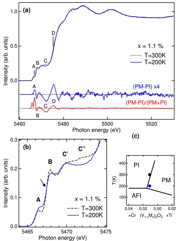
FIG. 4. (Color online) (a) V  $K$ -edge X-ray absorption spectra in a  $(V_{0.989}Cr_{0.011})_2O_3$  powder sample measured as a function of temperature in the PI (300 K, dashed line) and PM (200 K, solid line) phases in PFY mode; below, absolute and relative spectral differences (blue and red line, respectively); (b) pre-edge region; (c) corresponding points in the phase diagram.
