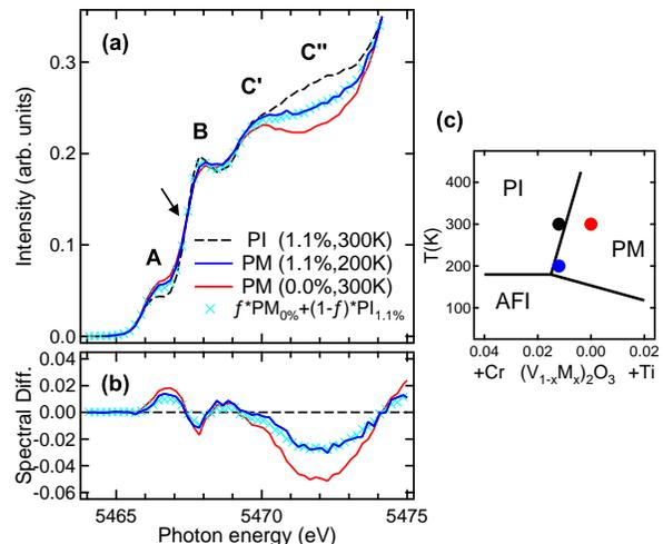
FIG. 7. (Color online) V-K pre-edge X-ray absorption spectra for a  $(V_{1-x}Cr_x)_2O_3$  powder sample as a function of temperature and doping level in PFY mode ( $x = 0, 0.011$  and  $T=200K, 300K$ ); crosses represent a linear combination of the room temperature spectra ( $PM_{0\%}$  and  $PI_{1.1\%}$ ) for a value of  $f = 0.54$ ; (b) PI-PM spectral differences; (c) corresponding points in the phase diagram.
