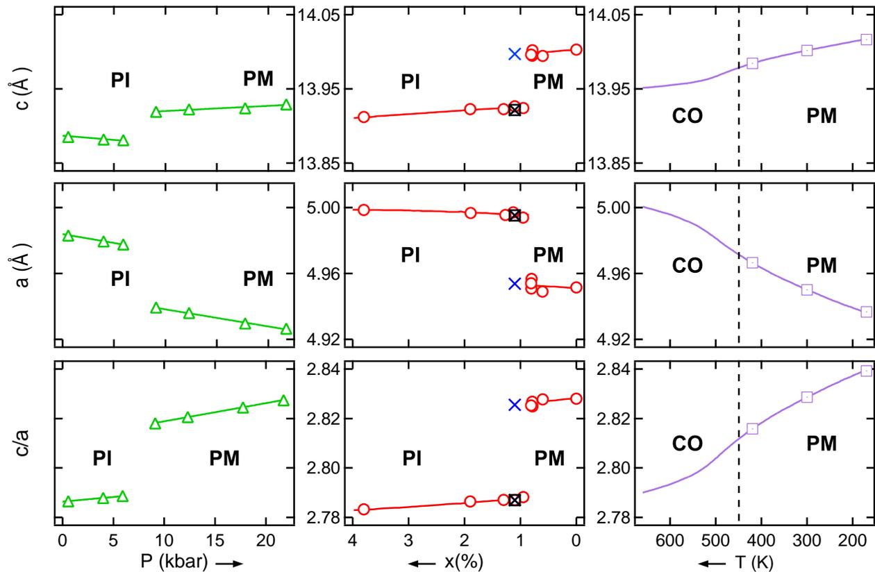
FIG. 11. (Color online) Lattice parameters as a function of pressure ( $x = 2.8\%$ , green triangles; the pressure scale refers to the  $x = 2.8\%$  doping), doping level (red circles, from Ref.<sup>1</sup>), and temperature ( $x = 0\%$ , purple square, from Ref.<sup>1</sup>). On the middle panel we also present the lattice parameters measured in a  $(V_{0.989}Cr_{0.011})_2O_3$  sample across the temperature-induced MIT in the PI (300K, black crossed square) and PM phases (200K, blue cross).
