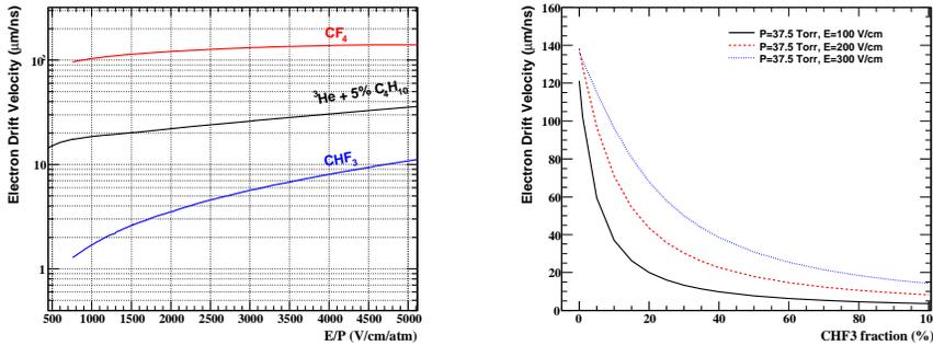
**Fig. 3.** Left: Electron drift velocity as a function of the electric field over the pressure in the chamber calculated with the Magboltz code in pure  $CF_4$ , in pure  $CHF_3$  and in  $^4He + 5\%C_4H_{10}$  mixture for comparison. Right: The electron drift velocity in a mixed of  $CF_4$  and  $CHF_3$  in 50 mbar as a function of the percentage of the last one for three different drift electric fields
