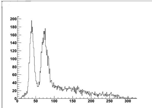
**Fig. 4.** X-ray calibration with  ${}^{109}\text{Cd}$  and  ${}^{55}\text{Fe}$  sources. We can see the 3.05 keV and the 5.9 keV lines. The second one broadened by the  $K_\beta$  6.4 keV not resolved.
