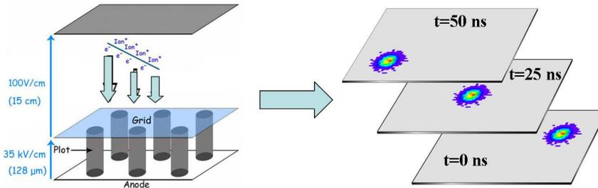
**Fig. 1.** Track reconstruction in MIMAC. The anode was read every 25 ns in the first version, now every 20 ns, giving the 3D track envelope from the consecutive number of images, defining the event. The drift velocity of the primary electrons, needed to recover the third dimension length, must be determined by an independent dedicated experiment.
