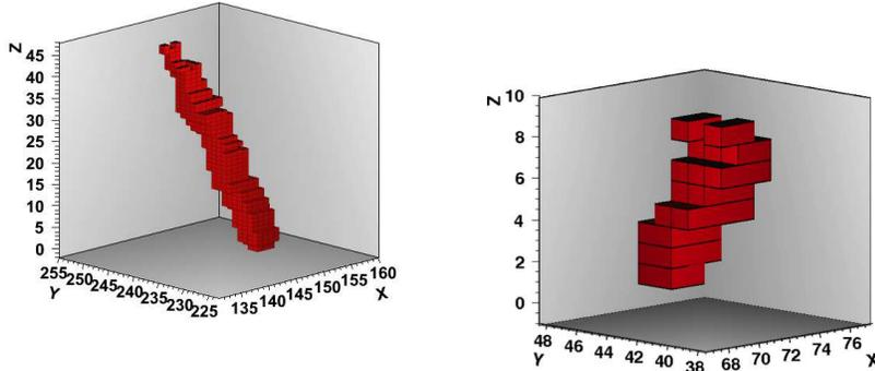
**Fig. 6.** Left: A 57 keV 3D proton track in  $CF_4$  plus 30%  $CHF_3$  in 50 mbar. Right: A 40 keV fluorine track in the same gas mixture
