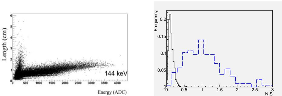
**Fig. 5.** : (Left): The length vs. ionization energy of all the raw events produced by the neutrons (144 keV) on  $C_4H_{10}$  and gamma rays produced on the target. (Right): The NIS, obtained as a sum of all the step deviations (every 20 ns) normalized by the energy, in black for recoils and in blue for electrons.
