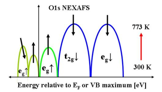
**Figure 4**. Schematic for the density of states for LaSrFeNi-oxide for temperatures from 300 K to 773 K as derived from VB PES [previous work in APL] and oxygen NEXAFS. The red arrow represents increasing temperature and. The direction of the arrow shows whether a structure increases/decreases in intensity, or shifts along the energy axis [6].
