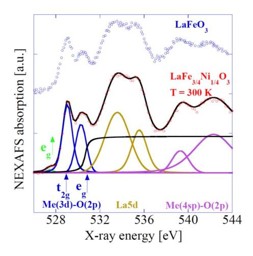
**Figure 1:** Oxygen 1s absorption spectrum of  $LaFe_{3/4}Ni_{1/4}O_3$  recorded at 300 K (bottom; open symbols are data points, solid line is least square fit) in ultra-high vacuum with suggested peak assignment and deconvolution into Voigt functions, and spectrum of LaFeO3 (top, open symbols) after Wu et al. [11].
