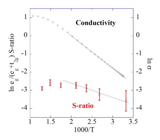
**Figure 3**: Arrhenius plot for the conductivity (top, right axis) and spectral ratio S (bottom, with error bars, left axis). Solid lines denote linear least square fits for the determination of the activation energy.
