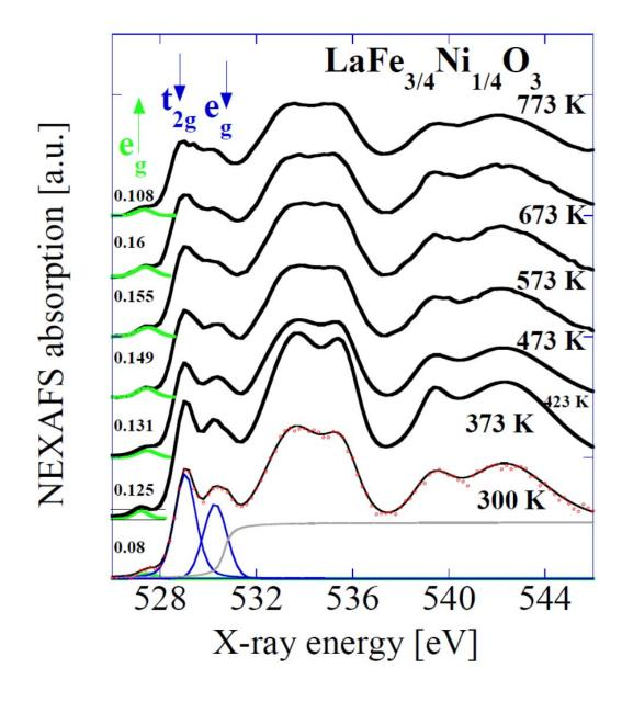
**Figure 2:** Oxygen 1s absorption spectra recorded at temperatures from 300 K to 773 K in ultra-high vacuum. Spectra are vertically offset by 1 unit for better comparison. Numbers on the left show the relative peak height of  $e_g\downarrow$ ; numbers on the right denote the temperatures.
