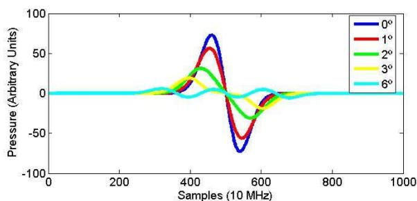
Figure 2. Pressure signal obtained at different angles for a three elements array.
