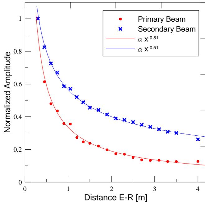
Figure 1. Amplitude of the primary and secondary signals as a function of the distance
