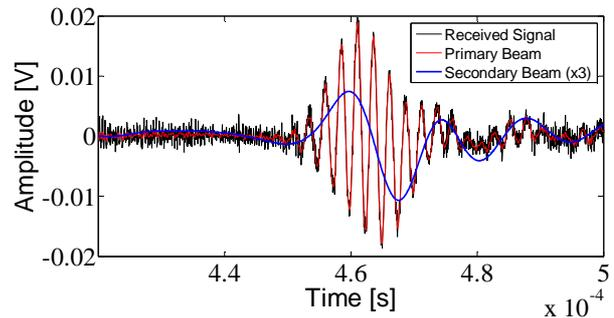
Figure 5. Example of a received signal and the primary and secondary beams obtained after applying the bandpass filters (the secondary beam has been amplified by a factor 3 for a better observation).
