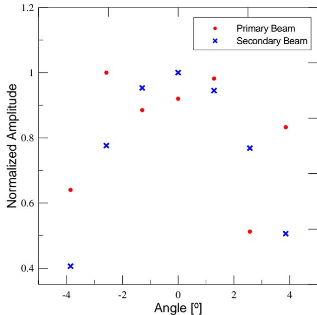
Figure 6. Directivity patterns of primary and secondary beam measured with the array.
