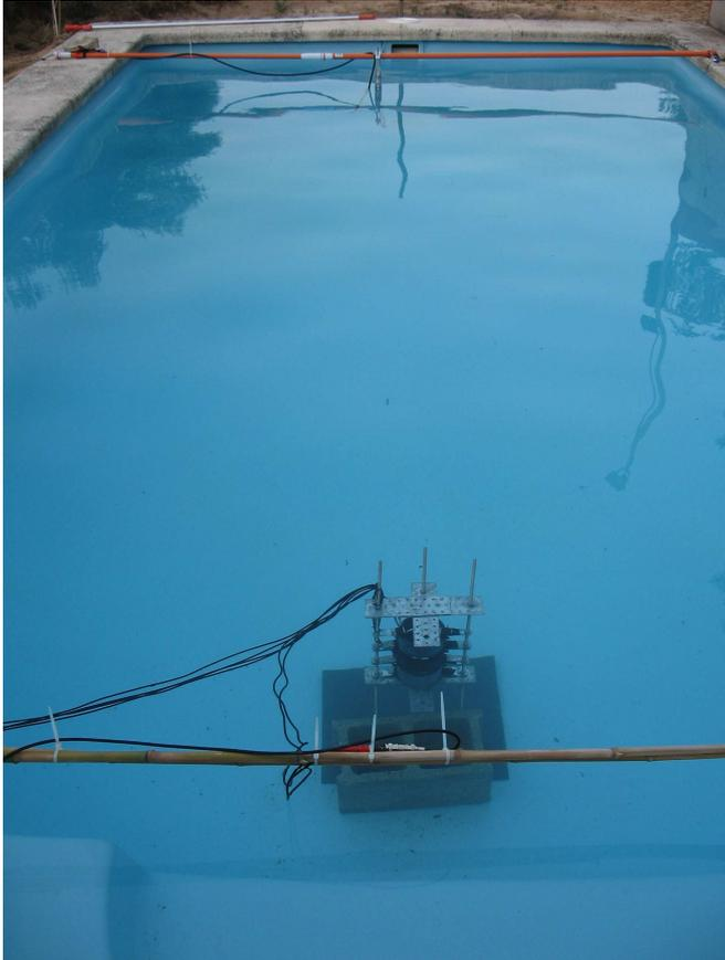
Figure 4. Picture of the pool during the data taking. The emitter array and the receiver (4.45 m apart) can be observed.
