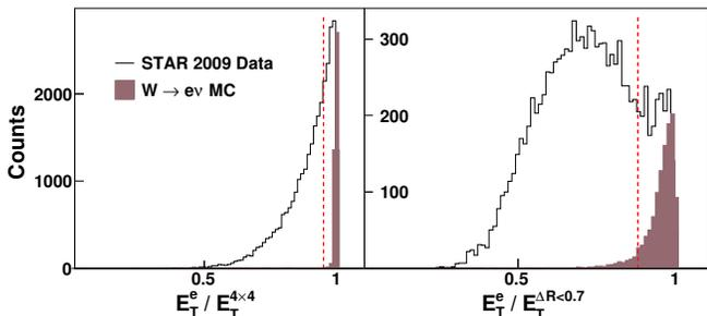
FIG. 3. (Color online) Distributions of the isolation ratios  $E_T^e/E_T^{4 \times 4}$  (left) and  $E_T^e/E_T^{\Delta R < 0.7}$  (right) used in  $e^\pm$  candidate selection.  $W \rightarrow e\nu$  MC shape distributions (arbitrary normalization) are shown as filled histograms for comparison with the data distributions. The vertical dashed lines indicate the placements of the cuts on these isolation ratios.
