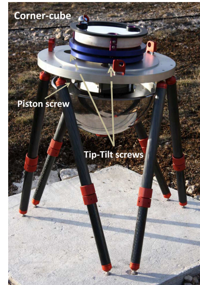
Fig. 6. Picture of the mount that carries one of the primary mirrors. With this hexapod we can position the mirror in rotation and translation. The carbon fiber legs insure a stability better than one micron.
