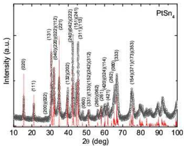
FIG. 2. Observed and calculated x-ray powder patterns of PtSn<sub>4</sub>. The open circles represent the observed data points and the solid line represent the calculated pattern. Representative (*hkl*) values are indicated.
