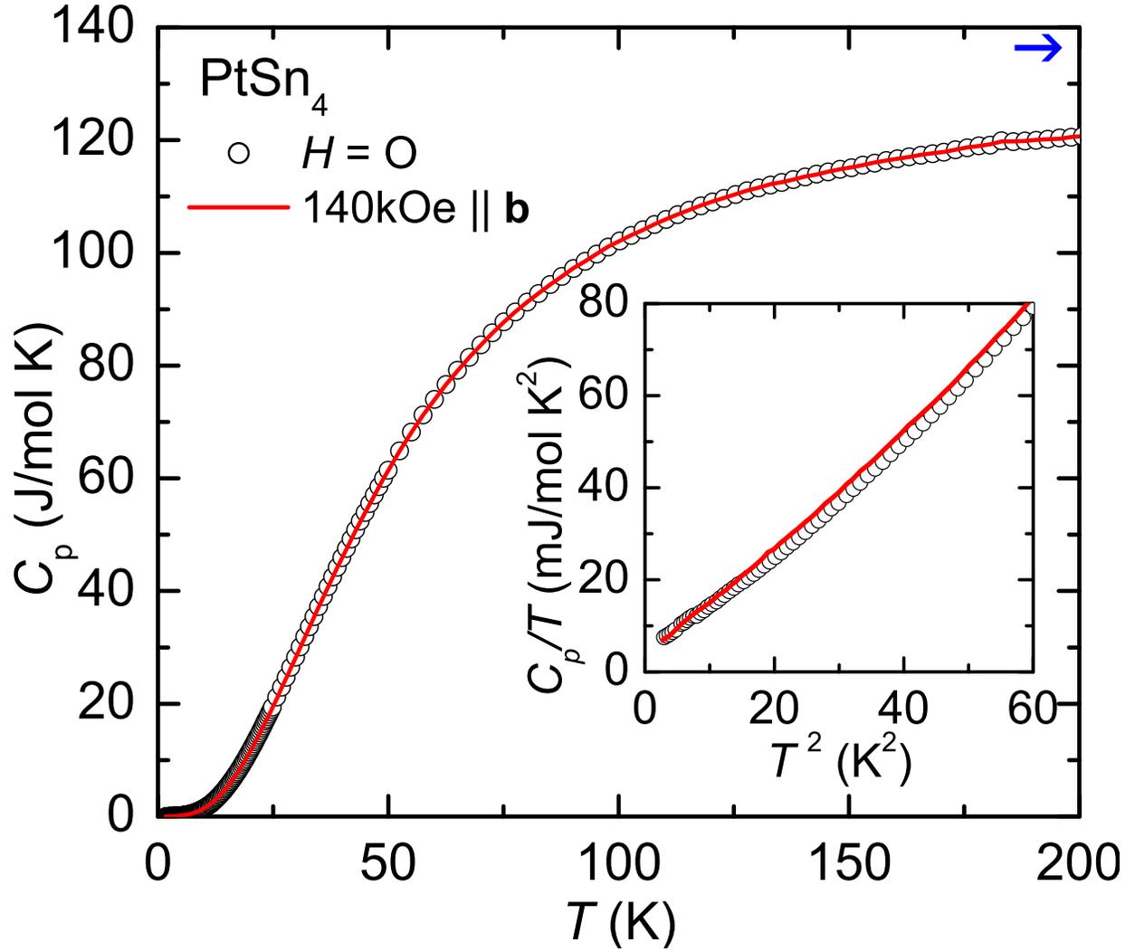
FIG. 3. Temperature dependence of the specific heat  $C_p$  of  $\text{PtSn}_4$  in  $H = 0$  (open circle) and 140 kOe (solid line). Inset:  $C_p/T$  vs.  $T^2$  plot. Horizontal arrow in the upper right corner indicates the classical limit of the Dulong-Petit law.
