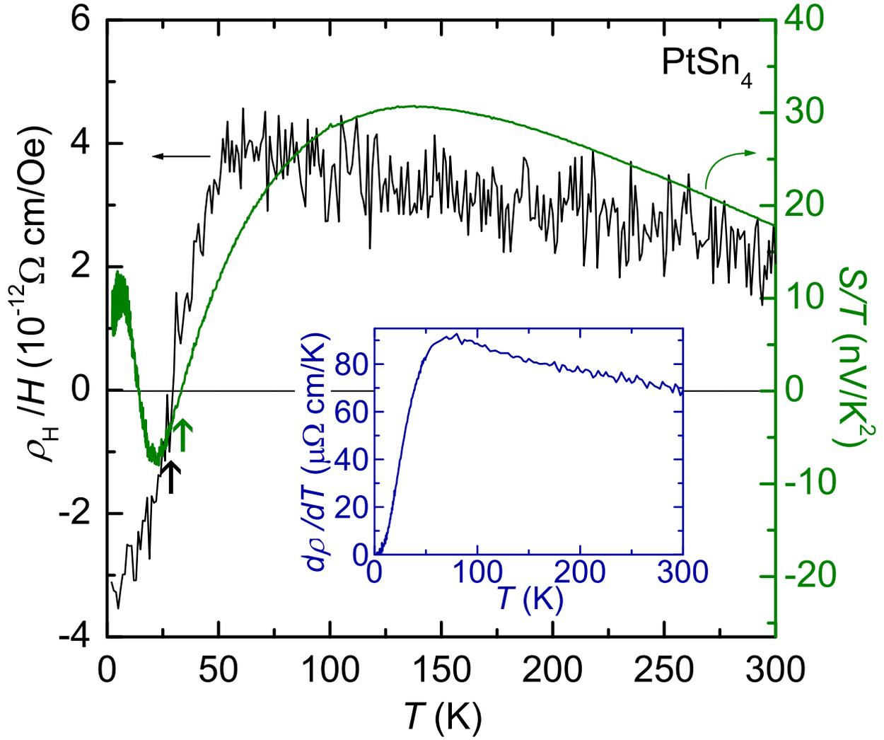
FIG. 10. Hall coefficient ( $R_H$ , left axis), TEP ( $S(T)/T$ , right axis), and resistivity ( $d\rho(T)/dT$ , inset) of PtSn<sub>4</sub> as a function of temperature. Vertical arrows indicate the sign reversal temperature corresponding to  $R_H = 0$  and  $S(T)/T = 0$ .
