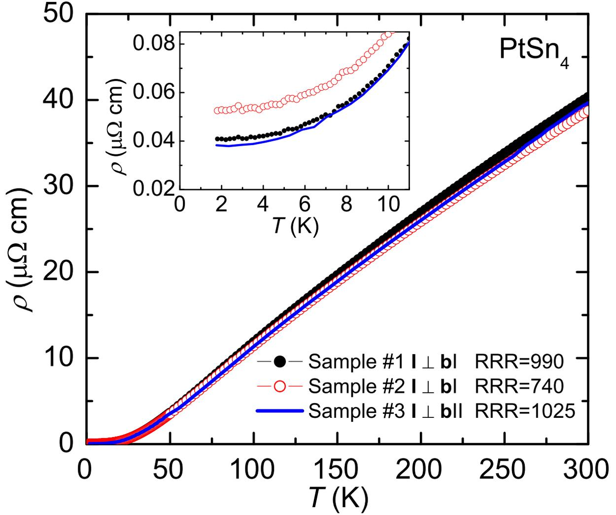
FIG. 5. Zero-field electrical resistivity of PtSn<sub>4</sub> for three samples. The current  $\mathbf{I}$  was applied parallel to the plane of longer axis ( $\mathbf{I} \perp \mathbf{bI}$ ) and shorter axis ( $\mathbf{I} \perp \mathbf{bII}$ ). Inset shows the low-temperature resistivity. For details see text.
