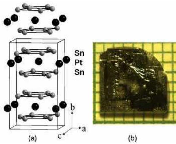
FIG. 1. (a) Crystal structure of PtSn<sub>4</sub>; along **b**-axis showing Sn-Pt-Sn layers. (b) Photo of a representative single crystal over a millimeter grid. The **b**-axis is perpendicular to the plate.
