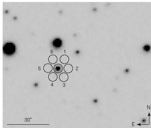
**Figure 1.** OPTIMA fibre bundle centred on V2069 Cyg. The ring fibres (1–6) are used to monitor the background sky simultaneously.
