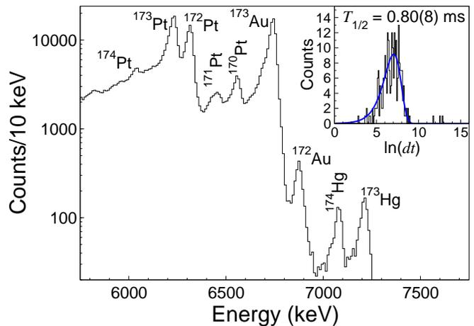
FIG. 1. (Color online) Spectrum showing all  $\alpha$  particles observed within 7 ms of the implantation of a recoil in the same pixel of the DSSD. The time distribution of detected  $\alpha$  particles identified with the decay of implanted  $^{173}\text{Hg}$  nuclei which have been correlated with their daughter activity ( $^{169}\text{Pt}$ ) is shown in the inset. The full blue line represents a fit to the data.
