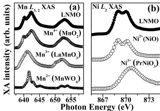
Figure 2. Mn  $L_{3,2}$  (a) and Ni  $L_2$  (b) XAS of LNMO, compared with reference spectra of compounds containing various valence states of Mn and Ni respectively, establishes that Mn exists as  $Mn^{4+}$  and Ni as  $Ni^{2+}$  in LNMO.
