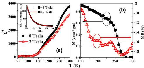
Figure 4. (Color online) (a) Dielectric constants at an applied frequency of 10 kHz in absence and presence of a magnetic field of 2 Tesla. The inset shows the absence of any DC magnetoresistance for applied magnetic fields upto 2 Tesla. (b) Temperature dependent magnetization (left axis, measured with  $H = 20$  Oe) and magnetodielectricity (right axis).
