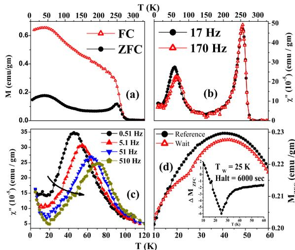
Figure 1. (Color online) (a) Field-cooled (FC) and zero-field cooled (ZFC) DC magnetization data, with an applied magnetic field ( $H$ ) of 20 Oe. (b) The imaginary parts of a.c. susceptibility ( $\chi''$ ), with  $H = 4$  Oe. (c) same as in (b), but focusing on the low-temperature region. (d) ZFC data with and without an intermediate wait ( $T_W$ ) at 25 K for 6000 seconds, showing distinct memory effects at  $T_W$  as illustrated in the inset with a difference plot.
