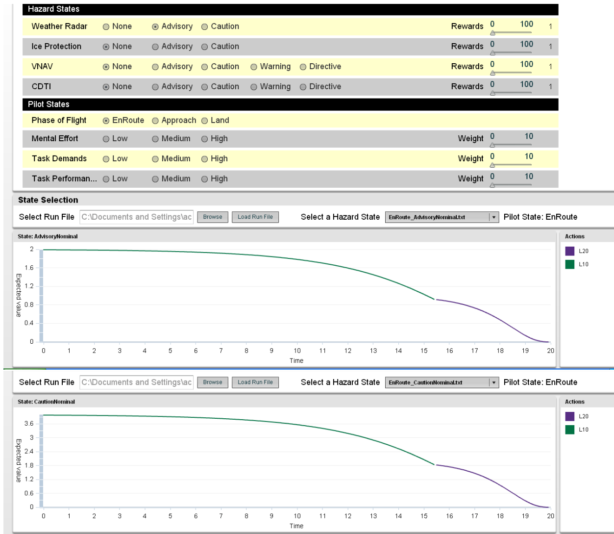
Figure 5: The ALARMS application. The top plot shows an Advisory for one hazard, the bottom plot was generated by changing the Advisory to a Caution (resulting in a doubling/rescaling of the y-axis).
