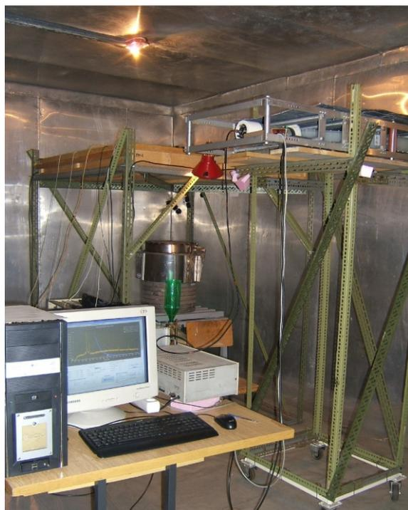
**Figure 2. Detectors in the underground laboratory (UL). The big plastic scintillator is positioned over the HPGe detector, seen in its lead shielding. The small plastic scintillator is in the front upper right corner. A hermetically sealed, 1 mm Al lining covering the entire UL, which enables the doubly filtrated ventilation system to sustain an overpressure of 2 mbar and keeps the radon concentration at an average level of some 10 Bq/m<sup>3</sup>, is also shown**
