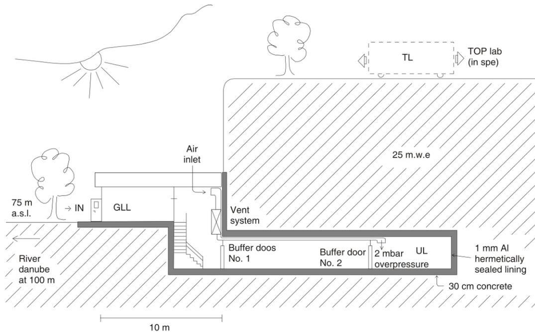
**Figure 1.** Cross-section of the low-level and CR laboratory at IOP, Belgrade, 44°49'N, 20°28'E, vertical rigidity cutoff 5.3 GV
