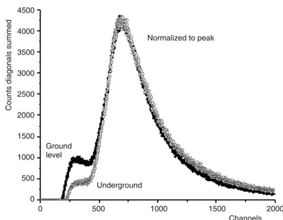
**Figure 9.** The sum spectra of two diagonals of the large plastic detectors in the UL and GLL. For comparison, the spectra are normalized for the peaks to coincide. Channel 650 now corresponds to the muon energy loss of 10 MeV. The integral of this peaked distribution is taken as the first approximation to the CR muon count by the large detectors
