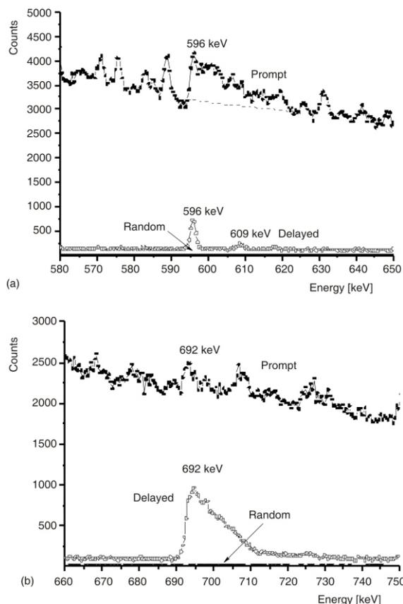
**Figure 5.** The spectrum of prompt, delayed, and random coincidences (practically negligible) containing: (a) the structure at 596 keV from inelastic fast neutron scattering on Ge-74 in the prompt spectrum, and the line of the same energy from slow neutron capture on Ge-73, in the delayed spectrum; (b) the structure at 692 keV from the inelastic scattering of fast neutrons on Ge-72, this time in the delayed spectrum, due to the finite lifetime of 444 ns at the excited state of 692 keV
