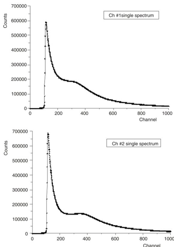
**Figure 8.** The spectra of two diagonals of the large plastic detector in the UL. Note that the peak of charged particle energy losses of 10 MeV, which corresponds to channel 320, is not separated from the low-energy tail of Compton scattered environmental gamma radiations. When summed, in coincidence they produce the spectrum from fig. 9
