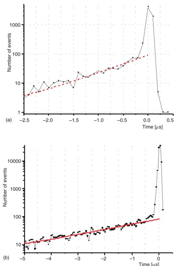
**Figure 12.** Time distributions of events that belong (a) to the structure of 692 keV, the slope of which yields 500(50) ns for the half-life of the state of this energy in <sup>72</sup>Ge and, (b) that of the annihilation line, which yields 2.24(9) s for the mean life of the muon
