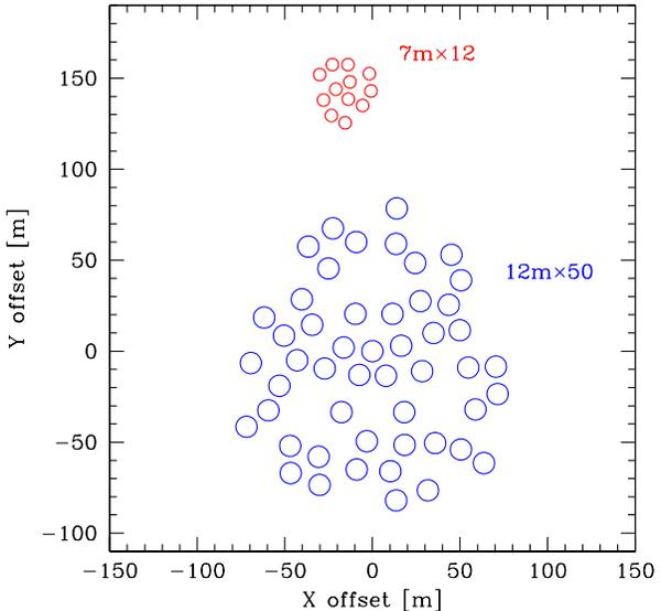
**Fig. 1.** The compact array configuration of  $12\text{m} \times 50$  and  $7\text{m} \times 12$  used in our mock observations. The projected positions on the UTM coordinate are shown with the symbol sizes representing the diameters of the telescopes.
