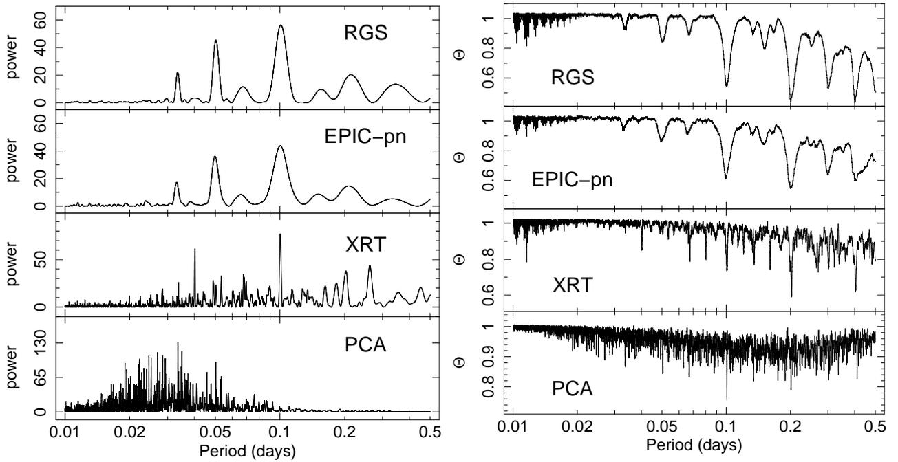
**Fig. 7.** Results of the Lomb-Scargle (*left*) and Phase Dispersion Minimisation (*right*) period analyses (see text) of the *XMM-Newton*/EPIC-pn (*top*), *XMM-Newton*/RGS (*second panel*), *Swift*/XRT (*third panel*) and RXTE/PCA (*bottom*) datasets.
