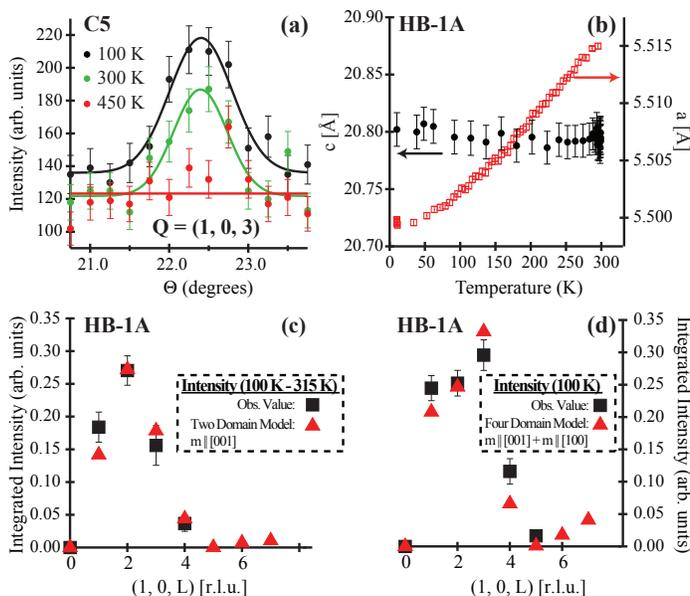
FIG. 4. (a) Rocking scans on a separate crystal showing the temperature dependence of the (1,0,3) peak above 300 K. (b) Temperature dependence of the  $a$ - and  $c$ -axis lattice parameters measured at the (2,0,0) and (0,0,4) reflections. Integrated intensities plotted as (c) 100 K with 315 K data subtracted and (d) the total scattering data at 100 K. Data is compared with two simple collinear spin models described in the text.
