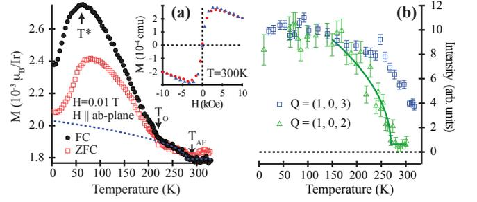
FIG. 2. (a) DC-magnetization data for Sr-327 with  $H = 0.01$  T aligned parallel to the *ab*-plane for both FC (solid symbols) and ZFC temperature sweeps (open symbols). Dashed line shows mean-field order parameter fit to the net moment from the 280 K transition. Inset shows  $M$  versus  $H$  sweep at 300 K. (b) Temperature dependence of the peak intensities at (1,0,3) and (1,0,2) magnetic reflections. Solid line is a power law fit to the (1,0,2) order parameter.
