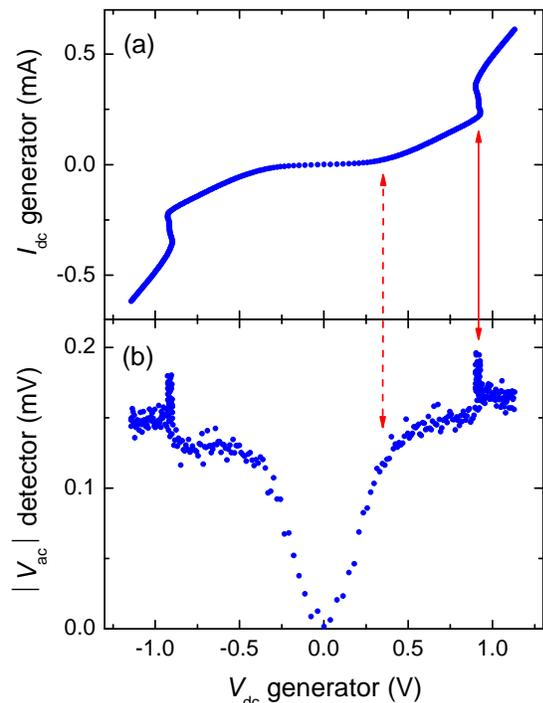
FIG. 6. (Color online). Radiation detection from junction #4 at  $T = 1.8$  K and  $H = 0$ . (a) The  $I$ - $V$  of the generator junction #4. (b) The signal of the detector junction. Appearance of a significant photon emission above the polaronic mobility edge in LMO (dashed line) and resonant enhancement of emission at the step (solid line) are seen.
