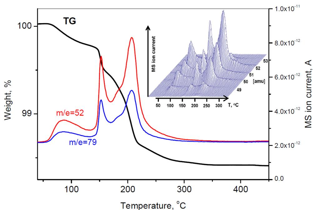
**Figure 3.** Thermogravimetric curve for  $\text{Li}_x(\text{C}_5\text{H}_5\text{N})_y\text{Fe}_{2-z}\text{Se}_2$  sample together with signals from the mass-spectrometer for the ions  $m/e=52$  and  $m/e=79$ . The insert shows the temperature evolution of  $m/e=49-53$  signals corresponding to different fragmentation of  $\text{C}_4\text{H}_4^+$ .
