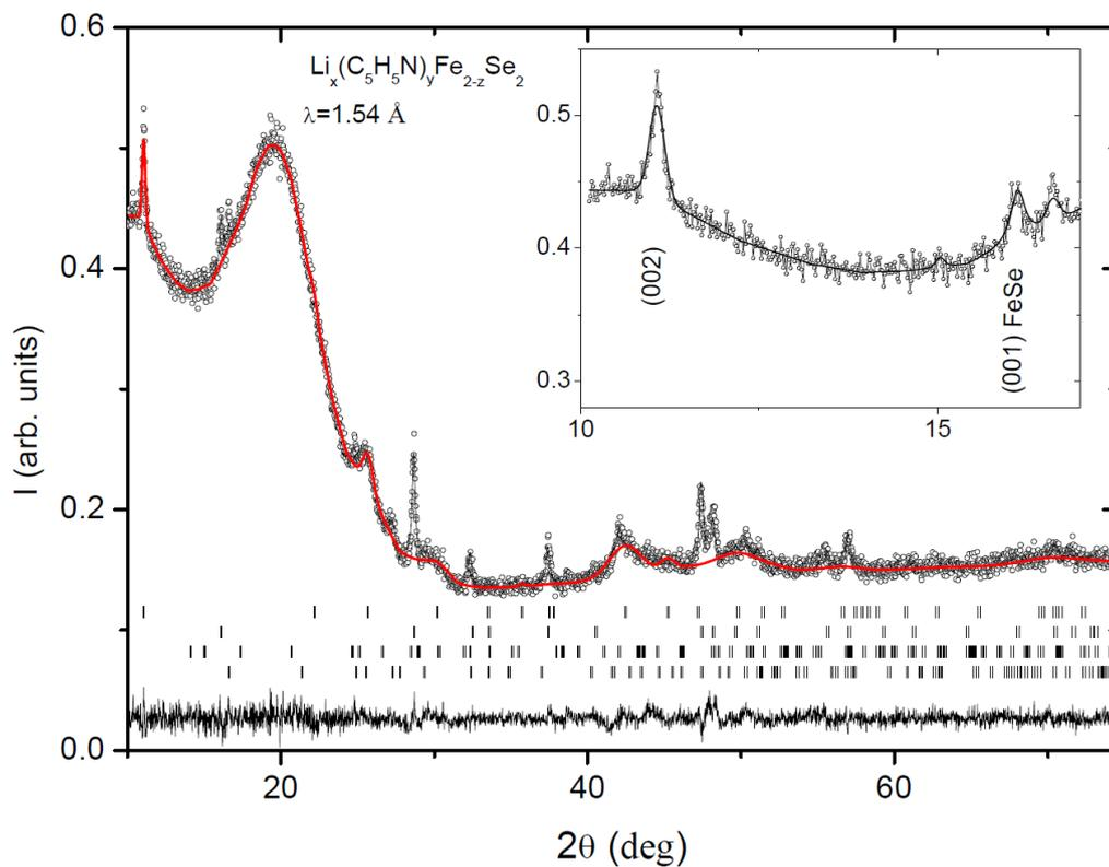
**Figure 2.** (a) X-ray powder diffraction pattern, the calculated profile and difference plot for  $\text{Li}_x(\text{C}_5\text{H}_5\text{N})_y\text{Fe}_{2-z}\text{Se}_2$  at 300 K. The rows of ticks show the Bragg peak positions for the 122, 11 FeSe and  $\text{Fe}_7\text{Se}_8$  phases, and the red line represents Le Bail mode refinement without structural fitting. (b) Fragment of the diffraction pattern at low  $2\theta$  showing (002) reflection of 122 phase and (001) belonging to 11 FeSe.
