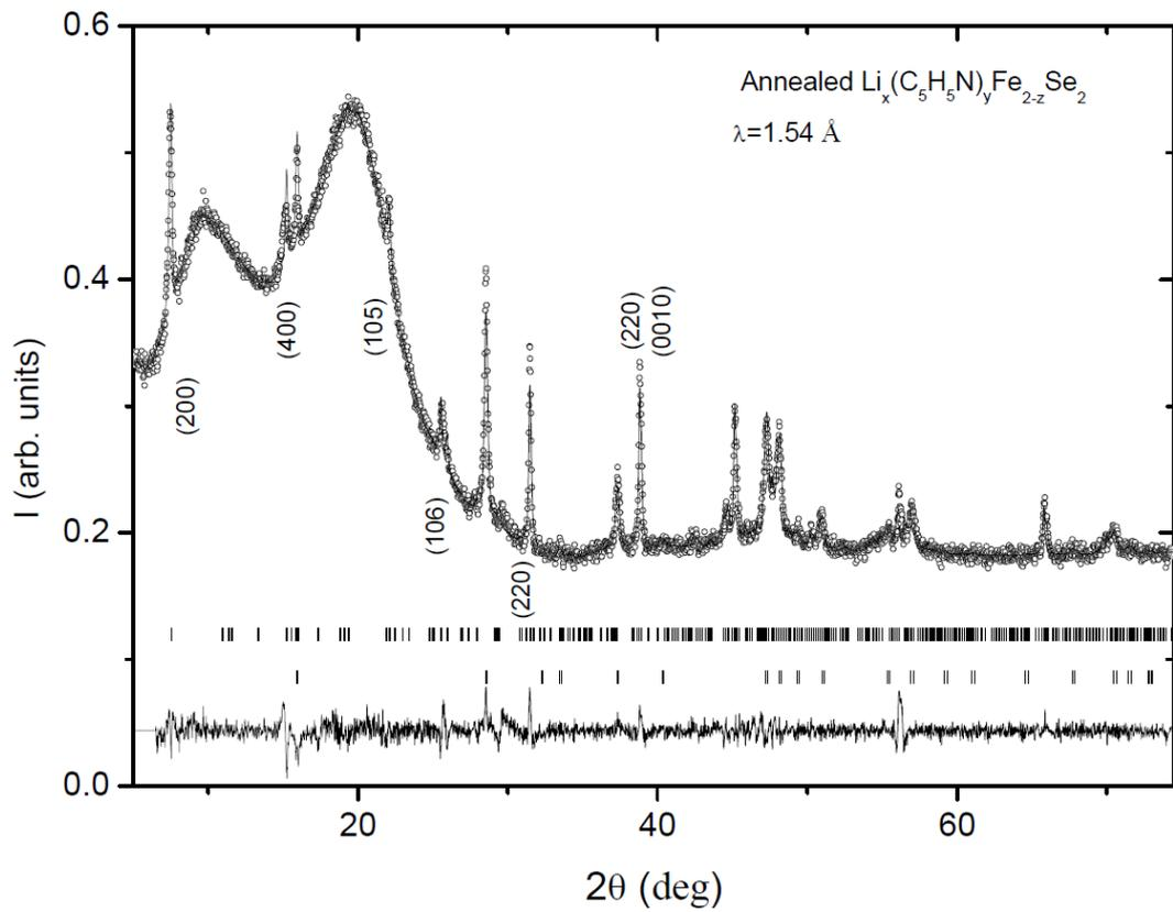
**Figure 5.** (a) X-ray powder diffraction pattern, the calculated profile and difference plot for the annealed sample of  $\text{Li}_x(\text{C}_5\text{H}_5\text{N})_y\text{Fe}_{2-z}\text{Se}_2$ . The main phase was refined in Lebeil mode in tetragonal cell with  $a = 8.00283$  and  $c = 23.09648 \text{ \AA}$ . The rows of ticks show the Bragg peak positions for the tetragonal P4 main phase and 11 FeSe. The first diffraction peaks of the main phase are labeled.
