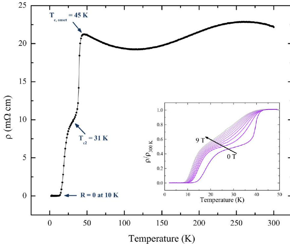
**Figure 6.** Temperature dependence of the electrical resistivity  $\rho$  of the as-prepared  $\text{Li}_x(\text{C}_5\text{H}_5\text{N})_y\text{Fe}_{2-z}\text{Se}_2$  sample. The insert shows magnetic field dependence of the resistivity.
