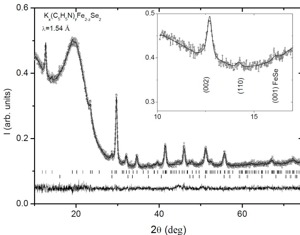
**Figure 1.** (a) X-ray powder diffraction pattern, the calculated profile and difference plot for  $K_x(C_5H_5N)_yFe_{2-z}Se_2$  at 300 K. The rows of ticks show the Bragg peak positions for the 122 and 11 phases. (b) Fragment of the diffraction pattern at low  $2\theta$  showing superstructure satellite (110). Its intensity corresponds to completely unoccupied Fe-vacancy site.
