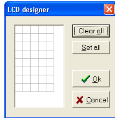
Figure 1. LCD designer - the LCD matrix has 7x5 cells
