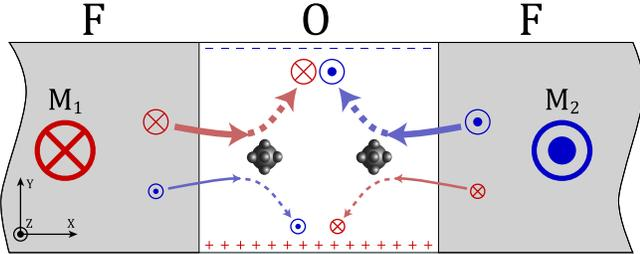
FIG. 2: Schematic illustration of AHE and SHE in MTJ due to spin-orbit scattering on impurities.  $\otimes$  and  $\odot$  denote the direction of magnetizations and electrons spins. The thickness of lines are proportional to Hall currents for the given projection of spin.
