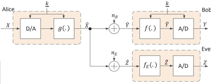
Fig. 1. The message  $X$  is observed at Bob and Eve through the transmitter, the AWGN channels with different noise variances, and their respective receivers with (possibly nonlinear) functions  $g(\cdot)$ ,  $f(\cdot)$ , and  $f_E(\cdot)$ . The sequence  $\underline{k}$  is a cryptographic key shared by Alice and Bob, which is assumed to be obtained by Eve immediately *after* she has recorded  $Z$ .
