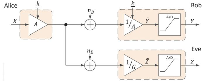
Fig. 2. Alice and Bob share a cryptographic key that determines the value of  $A$  at each time instance. Eve puts a (possibly variable) gain before her A/D to decrease the A/D erasures and/or overflows and hence increase the information leakage.
