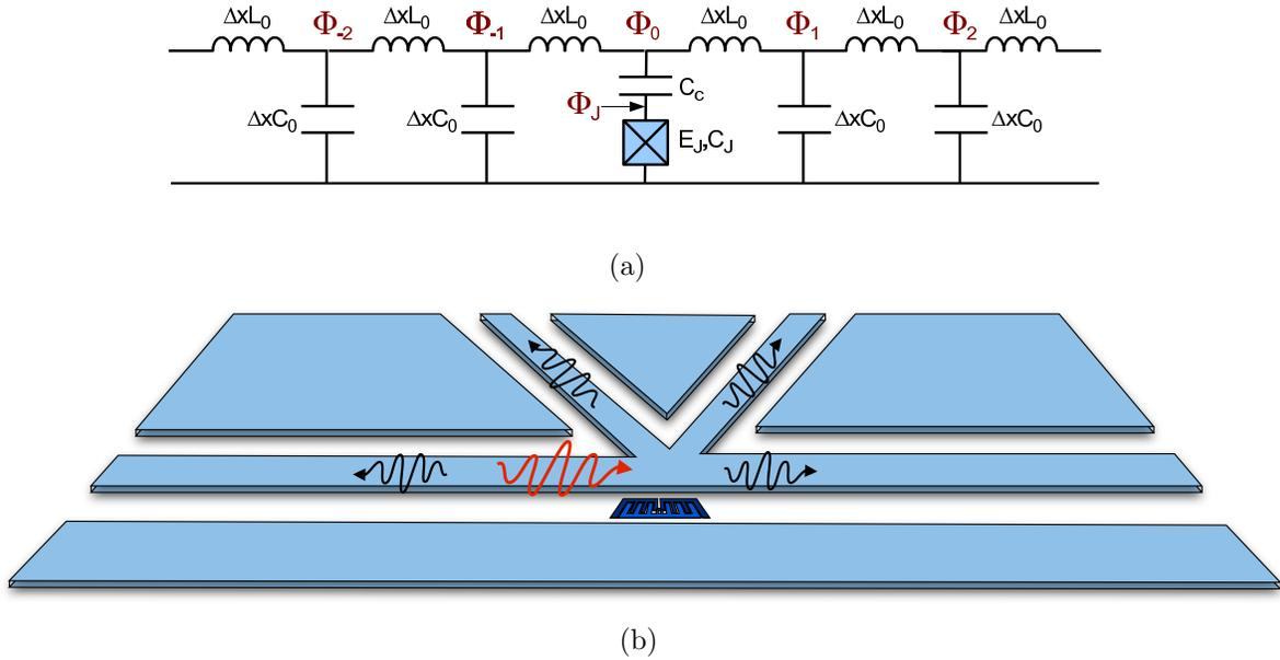
**Figure 2:** (a) Discretized circuit describing the interaction of a single Cooper-pair box with microwave photons propagating in an infinite transmission line. (b) Generalization of the input-output formalism to an arbitrary number of ports connected by an artificial atom.
