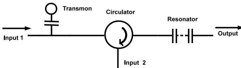
**Figure 6:** Schematic model of a transmon cascaded with a resonator. The circulator prevents the field reflected from the resonator to reach the transmon. Using input port 1(2), the output is the filtered transmitted (reflected) signal.
