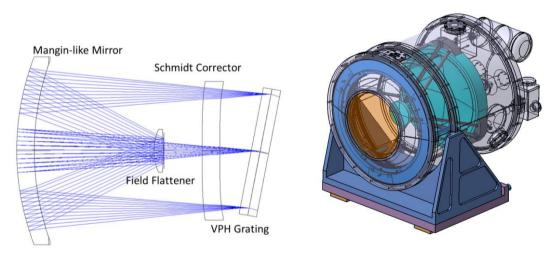
Figure 3. Optical Layout (left) and mechanical design (right) of the camera optics of the SpS.
