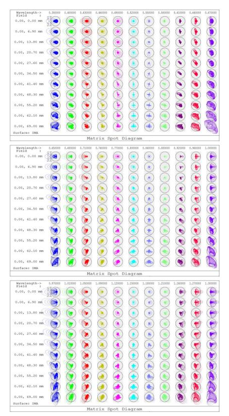
Figure 4. Spot Matrix (matrix field versus wavelength) in the "Blue" (top), "Red" (middle), and "NIR" (bottom). The circle corresponds to the dimension of the fiber on the detector (i.e. 50µm).
