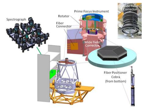
Figure 1. Overview of the Prime Focus Spectrograph (PFS) in the SUBARU telescope.
