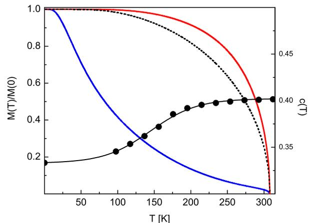
FIG. 8. The temperature dependence of magnetizations of surface sites  $M(T)$  for the  $A_2B$  ( $\sqrt{3} \times \sqrt{3}$ ) surface model. Solid blue and red lines denote magnetization of site A and B, respectively. Dotted black line denote bulk sublattice magnetization. Black circles show MC results for the temperature dependence of the concentration of surface Cr ions occupying site B. The solid black lines is the best fit to MC data.
