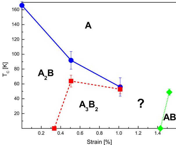
FIG. 6. MC transition temperatures for different orderings as a function of tensile strain. Blue circles, red square and green rhombi denote transition temperatures below which  $A_2B$  ( $\sqrt{3} \times \sqrt{3}$ ),  $A_3B_2$  ( $\sqrt{3} \times \sqrt{7}$ ), and AB ( $1 \times 2$ ), orderings respectively set in. Lines connecting the points are guides to the eye.
