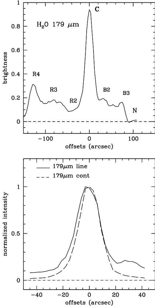
**Fig. 3. Upper panel:**  $\text{H}_2\text{O}$   $179\ \mu\text{m}$  intensity cut along the L1448 flow, at PA  $164^\circ$ . The normalized intensity is integrated over a width of  $30''$  perpendicular to the cut. The location of the C(N) source is taken as the reference for the offsets. **Bottom panel:** normalized intensities of the  $179\ \mu\text{m}$   $\text{H}_2\text{O}$  line and continuum, along the same cut direction as above.
