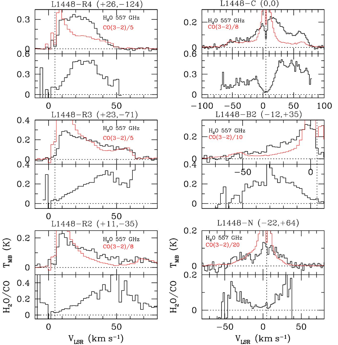
**Fig. 5.**  $\text{H}_2\text{O}$   $1_{10-1_{01}}$  (black) and  $\text{CO}(3-2)$  (red) line profiles at selected outflow positions.  $\text{CO}$  line profiles, convolved to the  $\text{H}_2\text{O}$  spatial resolution, have been scaled to match the  $\text{H}_2\text{O}$  line wings and the corresponding scaling factor is indicated in each plot. At the bottom of each spectrum, the relative  $\text{H}_2\text{O}/\text{CO}$  intensity ratio is plotted as a function of velocity.
