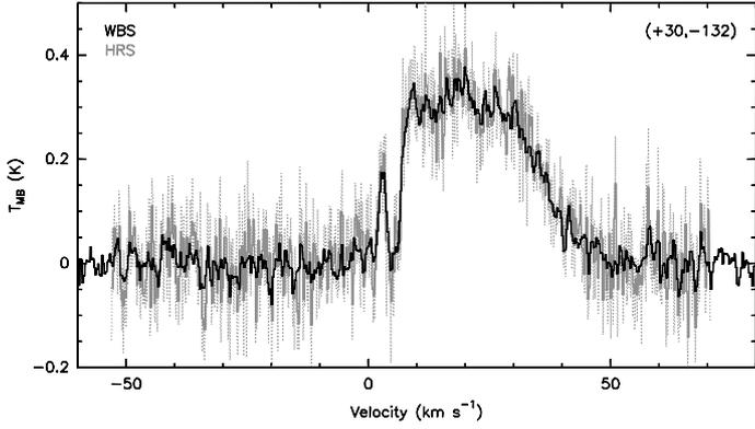
**Fig. 1.** Comparison between a WBS and HRS spectrum at a representative position in the outflow (offsets with respect to L1448-C are indicated). Full black lines show the WBS data, while the gray dotted and full lines show the HRS data before and after smoothing to the WBS resolution, respectively.
