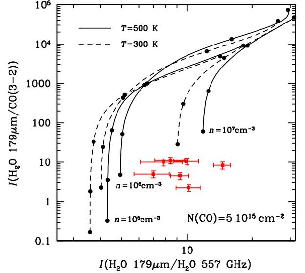
**Fig. 9.** Diagnostic diagram employing the  $\text{H}_2\text{O} 179 \mu\text{m}/557 \text{GHz}$  vs the  $\text{H}_2\text{O} 179 \mu\text{m}/\text{CO}(3-2)$  intensity ratios. Theoretical LVG predictions are plotted for the same parameters as in Fig. 8. The plot assumes a fixed  $N(\text{CO})$  column density of  $5 \cdot 10^{15} \text{cm}^{-2}$  (see text for details). Data points refer to intensities measured in a beam of  $38''$ , equal to the beam of the 557 GHz observations.
