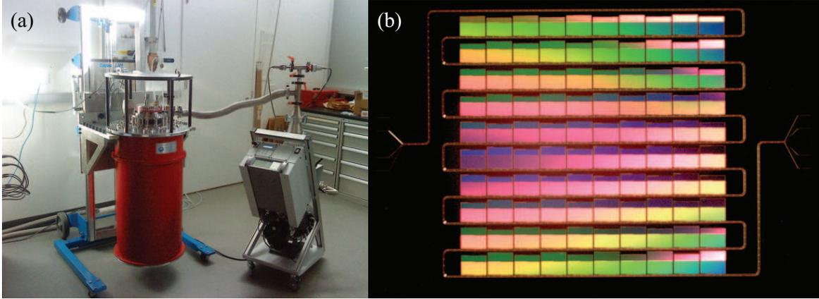
Figure 1. The MAKO instrument. (a)  $^3\text{He}$  measurement cryostat with a stable base temperature of 250 mK. (b) First generation 100 pixel test array. Here the single transmission line is coupled to the inductive meander portion of each pixel and is used to read out the entire array. For this initial design the capacitor occupies  $\sim 35\%$  of the pixel area.
