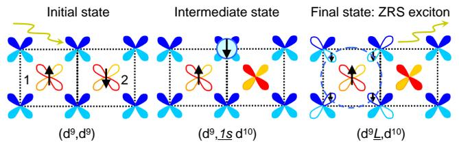
FIG. 2: Schematic illustration of how a ZRS exciton is created in the RIXS process at the oxygen  $K$ -edge. See text for detailed explanations. Unoccupied states are depicted with empty orbitals.
