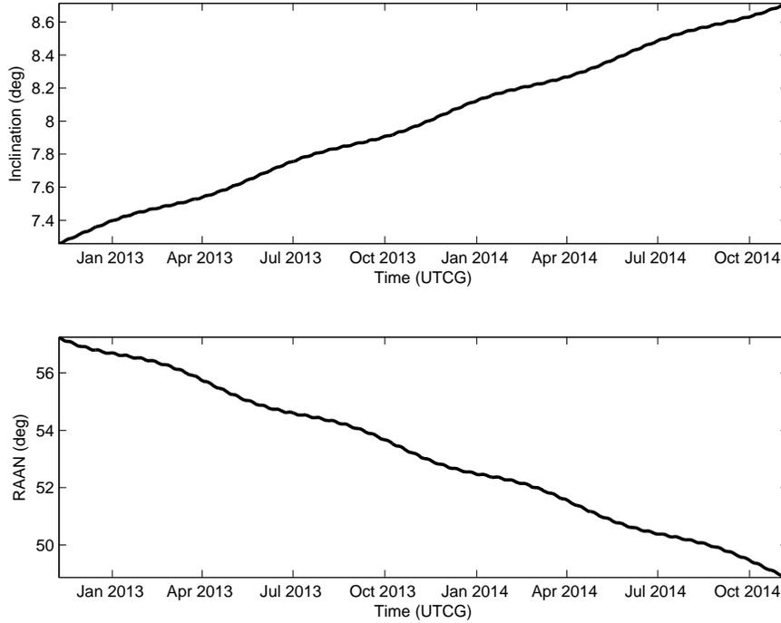
Fig. 1: Orbital evolution of SIGSO satellite under perturbations (Ma et al. 2011b).
