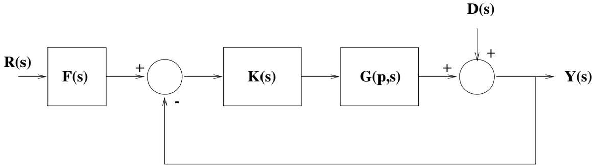
Figure 1: Two degree of freedom feedback system
