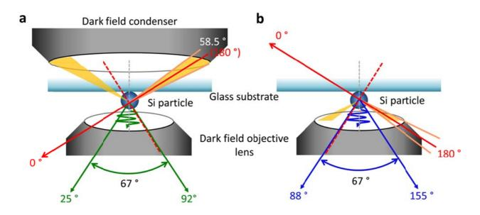
Figure S1. Detailed schematic illustration of the forward (a) and backward (b) scattering measurements.
