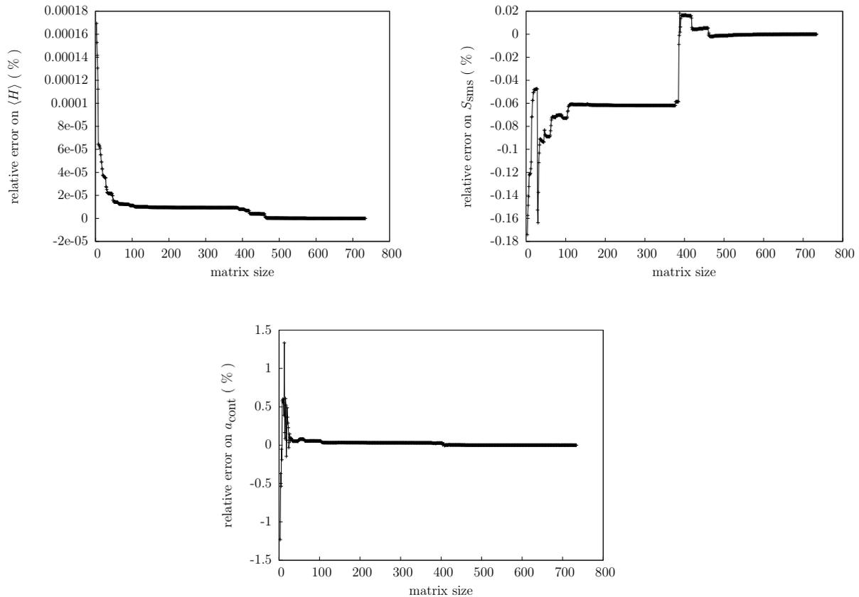
**Figure 9.** Progressive deconstraint of the many-electron wave function. The three curves illustrate the relative difference between the CI calculation and the partially deconstrained problem for respectively the total energy, the specific mass shift parameter and the hyperfine contact parameter for the ground state  $1s^2 2s^2 S$  of neutral lithium.
