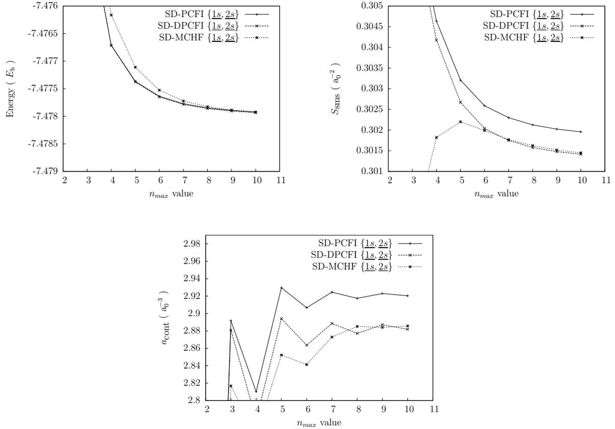
**Figure 3.** Convergence of the absolute total energy, the specific mass shift and the hyperfine contact parameters for the ground state of neutral lithium. The agreement found between the SD-MCHF and SD-PCFI curves for the total energy is not observed for the two other properties. We recover the consistency with the traditional method by deconstraining the wave function (SD-DPCFI).
