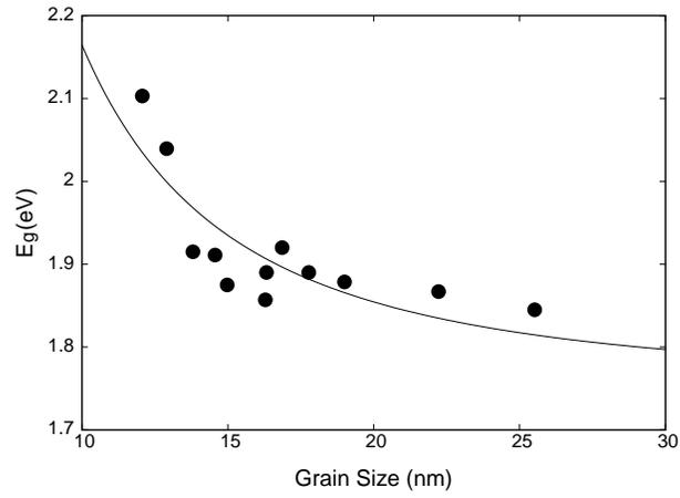
Figure 4: Variation of band-gap with grain size.
