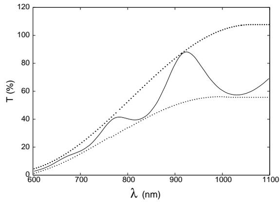
Figure 5: The transmission spectra of a SnS thin film with envelopes used to calculate the film's refractive index.
