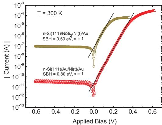
FIG. 2. Electrical (I-V) characterization of the devices on n-Si(111) with two different Schottky barrier heights at room temperature. The active device area was 150  $\mu\text{m}$  in diameter. The straight lines were fitted using the thermionic emission theory as described in the text.
