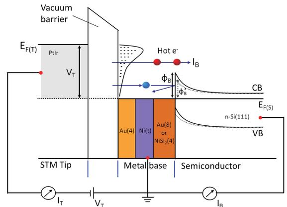
FIG. 1. Schematic layout and energy band diagram of a BEEM experiment. A PtIr tip is used to inject hot electrons over the vacuum barrier, in a Au(NiSi<sub>2</sub>)/Ni/Au base. The transmitted electrons are then collected in an n-Si(111) semiconductor. Au and NiSi<sub>2</sub> layers on n-Si(111) give rise to two different SBHs  $\phi_B$  or  $\phi'_B$  as depicted.
