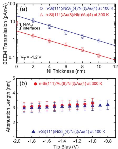
FIG. 5. (a) Normalized BEEM transmission as a function of Ni thickness at  $V_T = -1.2$  V for both the Schottky interfaces. (b) Variation of the attenuation length in Ni with energy for both the Schottky interfaces.
