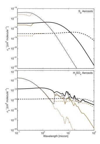
Fig. 1.— Extinction cross sections (black lines) and scattering cross sections (orange lines) of  $H_2SO_4$  and  $S_8$  per molecule in the condensed phase. The dotted, solid, and dashed lines are cross sections for the mean particle diameter of 0.1, 1, 10  $\mu$ m, respectively. The size distribution of aerosol particles is assumed to be lognormal with a dispersion  $\sigma = 2$ .
