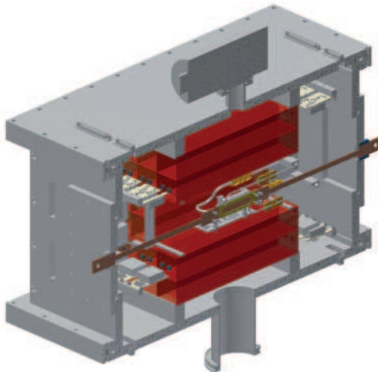
**Figure 1.** An artist view of the VIP2 experimental setup. In the middle the copper conductor and the x-ray detectors are installed. Plastic scintillators with solid state photodetector readout acting as active shielding (see fig.3) are surrounding this inner part.
