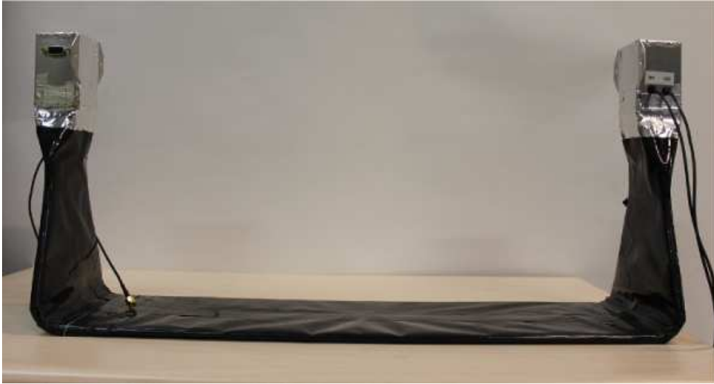
Figure 10: Photograph of one pGAPS scintillator paddle. The paddle includes a 50 cm long BC-408 plastic scintillator slab, two acrylic light guides, a light-tight wrapping, and fast PMT assemblies mounted on each end.
