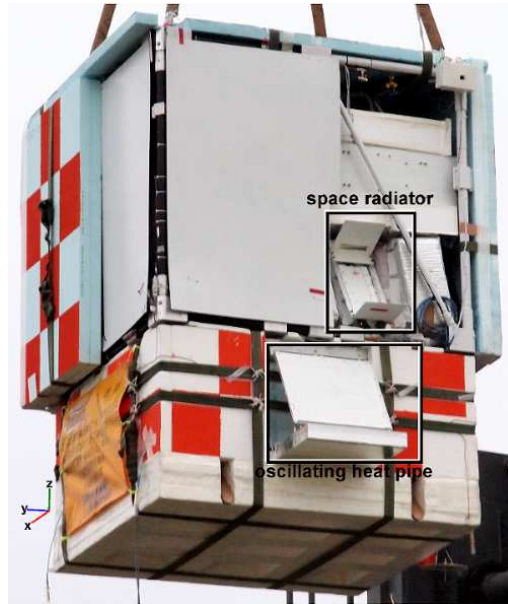
Figure 8: Space radiator and oscillating heat pipe shown on the (flight ready) pGAPS payload.
