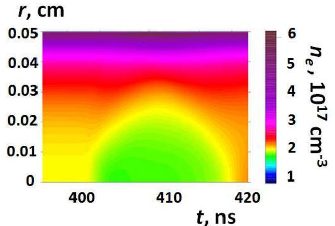
FIG. 2: Capillary discharge dynamics with laser heater: The distribution of the electron density in units of  $10^{17} \text{ cm}^{-3}$  in the  $(r, t)$  plane.
