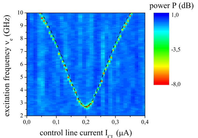
FIG. 4: Fluxon response on the microwave excitation applied to the flux qubit. Color scale corresponds to the detected power. Measured power  $P$  relates to the power at the fixed frequency offset  $+50$  kHz from the fluxon mean oscillation frequency  $\nu_f$ . Every point consists of 10 averages with video filter bandwidth of 1 Hz. The flux qubit spectrum can be clearly seen as the red-yellow curved trace. The black dashed line depicts the corresponding fit of the flux qubit.
