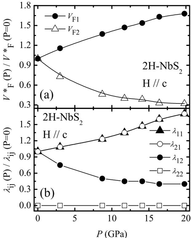
FIG. 5: Pressure dependence of the renormalized Fermi surface velocities  $v_{Fi}^*(P)/v_{Fi}^*(0)$  (a) and of the electron-phonon coupling parameters  $\lambda_{ij}(P)/\lambda_{ij}(0) = \rho_j(P)$  (b) for both subgroups of electrons in 2H-NbS<sub>2</sub>. Lines simply join points and are a guide to the eyes.
