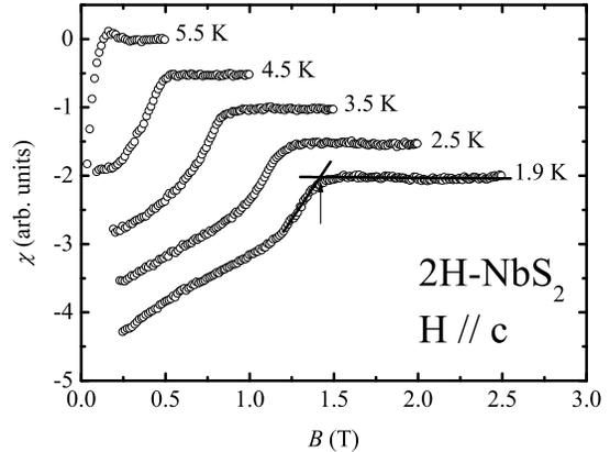
FIG. 3: Variation of the susceptibility of a 2H-NbS<sub>2</sub> sample as a function of the magnetic field, for a pressure of 3 GPa and for several temperatures. The arrow and the lines show the way we used to extract the corresponding value of  $H_{c2}(T)$ . Note that the transition width significantly increases with magnetic field. Other criteria for determining the transition temperature, such as midpoint or lower part of the transition region, lead to similar  $H_{c2}(T)$  curves.
