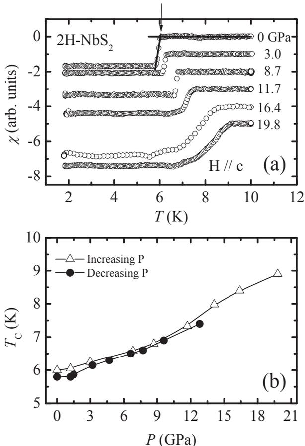
FIG. 2: (a) Variation of the susceptibility of a 2H-NbS<sub>2</sub> sample as a function of temperature and for several applied pressures. The arrow and the lines show the way we used to extract the corresponding value of  $T_c$ . (b) Critical temperature as a function of the applied pressure. Triangles and full circles correspond to increasing and decreasing pressure, respectively. Lines are a guide to the eye and simply join data points. Saturation is eventually expected above 20 GPa.
