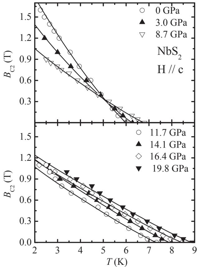
FIG. 4: Temperature dependence of the upper critical field  $H_{c2}(T)$  as a function of pressure (empty and filled symbols). Fits to the model explained in the text are shown as lines. Note the decrease in the upper critical field until 8.7 GPa (upper panel), which ceases above this pressure (lower panel).
