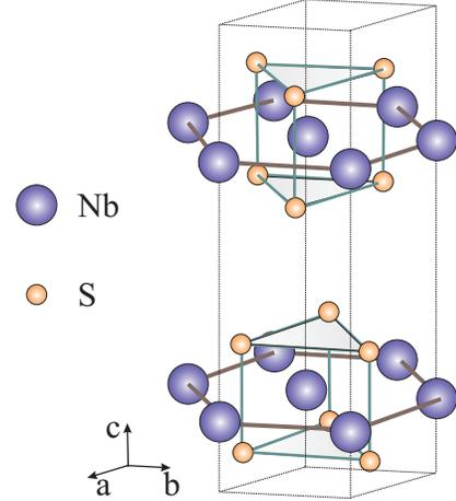
FIG. 1: Structure of 2H-NbS<sub>2</sub>. The niobium atoms are surrounded by sulphur atoms following a trigonal prismatic coordination. The S-Nb-S layers that make up each packet are covalently bound. The coupling between pairs of packets is dominated by van der Waals forces. The lattice parameters are  $a = 3.321\text{\AA}$ ,  $b = 5.751\text{\AA}$  and  $c = 11.761\text{\AA}$  [26].
