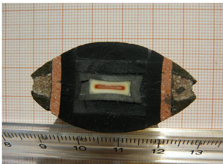
**Figure 1.** (colour online) Cross-section of the pressure pellet containing a polycrystalline sample of coesite synthesised at  $P= 5.5 \text{ GPa}$  and  $T=1000 \text{ C}$ .
