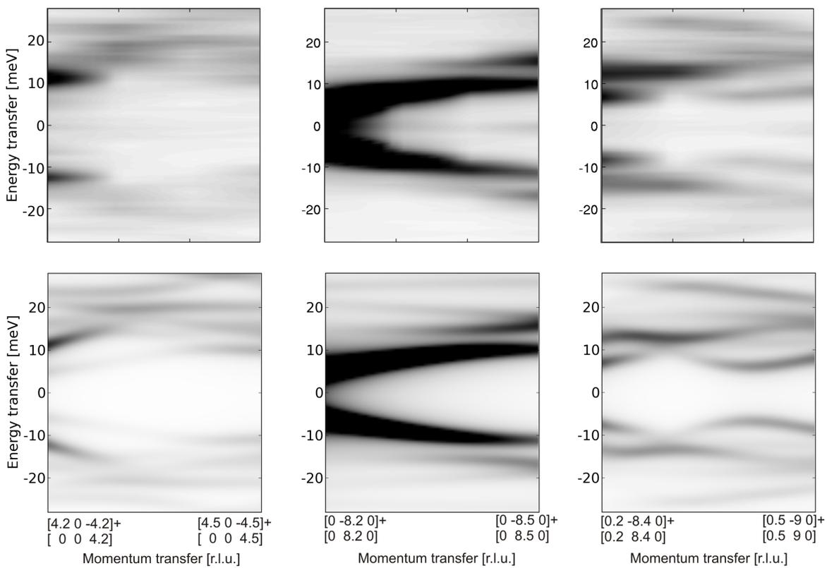
**Figure 4.** Experimental IXS intensity maps (first row) from coesite crystal together with theoretical intensity maps (second row) along the indicated directions. See text for further details.
