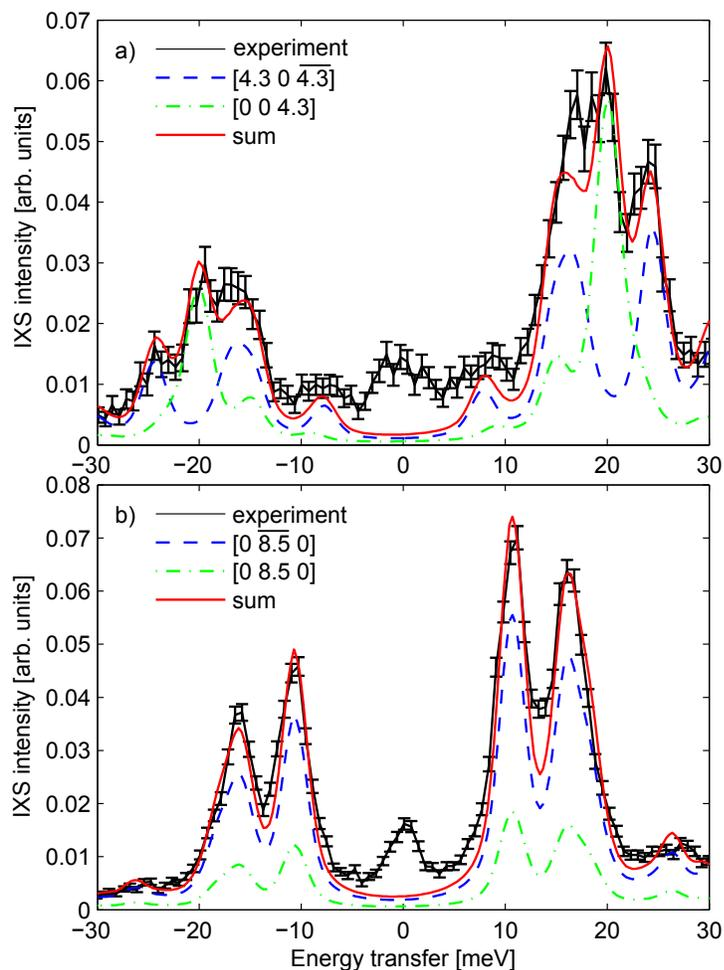
**Figure 3.** (colour online) Experimental (black points with errorbars) and theoretical (red line) IXS spectra from coesite crystal. The theoretical spectra are the weighted sum of the two crystalline orientations: domain 1 - 75% (blue dashed line), domain 2 - 25% (green dotted dashed line). Theoretical intensities were convoluted with the experimental resolution function and the energy transfer was scaled by 1.045.
