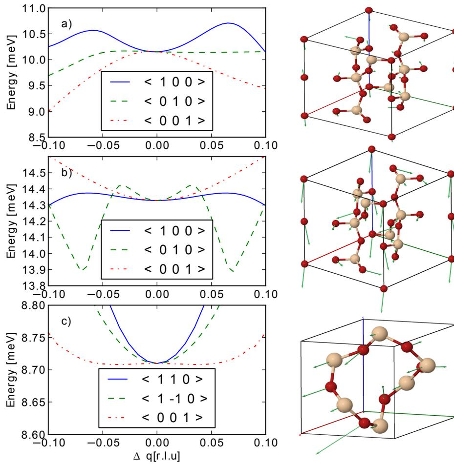
**Figure 6.** (colour online) a) Dispersion relations along the main crystallographic directions through the critical point (0.87 0.69 0.42) and the displacement pattern (primitive cell) of the atoms at this saddle point contributing strongly to the first peak in the VDOS of coesite. b) Dispersion relations and displacement pattern at the Y point (1 0 0) in coesite. c) Orthogonal dispersion relations and displacement pattern at the L point (1/2 0 1/2) in  $\alpha$ -quartz.
