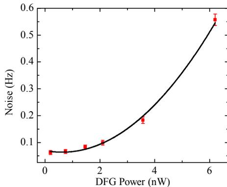
FIG. 6: Quadratic behaviour of noise in detector D2 as a function of DFG source power.
