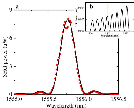
FIG. 7: **a**, Second harmonic generation spectrum. Solid line: fit of the data. **b**, Zoom of fit, showing the predicted intensity of SHG at 1551 nm.
