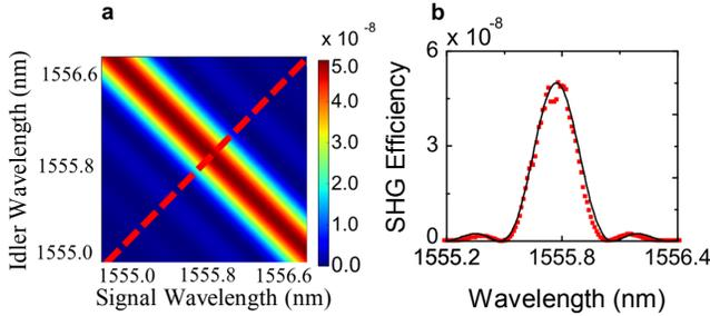
FIG. 3: **a**, Calculation of the waveguide efficiency taking into account the quasi-phase matching conditions. **b**, Measured values for the efficiency of second harmonic generation (red points) compared to the theoretical prediction (solid line), showing an almost ideal phase matching of the PPLN waveguide.
