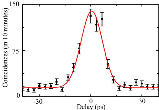
FIG. 4: Temporal overlap of input signals at the waveguide measured by introducing a delay between the photons' arrival times. The fit (solid line) gives a FWHM 14.8 ps, which corresponds to a convolution of two pulses of 10 ps from our laser. The spectra of the SPDC and of the DFG are, respectively, 1.2 nm and 0.8 nm, corresponding to 6.76 ps and 10.03 ps. This indicates that to within the resolution of our measurement, our photons are close to being single mode.
