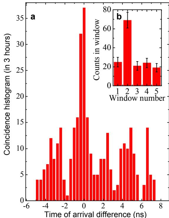
FIG. 5: **a**, Coincidence histogram between D1 and D2 showing strict time correlation between the heralding upconverted photon and the 807 nm photon. The spread of the coincidence peak is mainly dominated by detector jitter. Side peaks are due to the periodicity of the laser. **b**, Bar chart histogram, obtained by integrating the two central bins of each peak.
