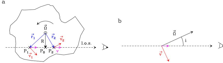
**Fig. 1.** **a** Projection of the rotation velocity of an object in solid-body rotation along the line of sight, for the particular case where the rotation axis is orthogonal to the line of sight, viewed from the top. **b** Configuration when the rotation axis has an inclination  $i$  to the line of sight, viewed from the side.
