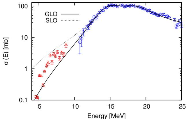
FIG. 10. (color online). Deduced total cross sections from this work, and GDR cross section data from above the particle separation threshold [24], triangles and circles respectively. The GDR data has been fitted to both a standard and generalized Lorentzian form. For the case of the GLO form, an enhancement is observable upon the extrapolated tail of the GDR.
