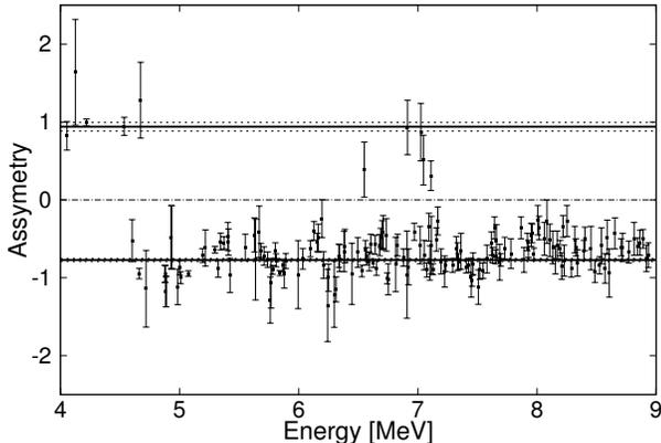
FIG. 2. Azimuthal efficiency corrected count rate asymmetries for all states in  $^{76}\text{Se}$  observed at the HI $\gamma$ S facility. A positive asymmetry corresponds to a positive parity state, and a negative asymmetry to a negative parity state. The deviations from the expected values of  $\pm 1$  are due to the finite opening angles of the detectors and limited statistics.
