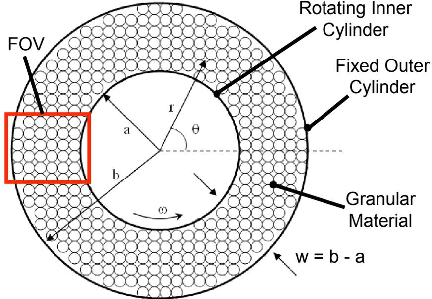
FIG. 6. The Taylor-Couette Geometry ( $a$  = inner cylinder radius,  $b$  = outer cylinder radius,  $w$  = width of shear region,  $r$  = radial distance,  $\theta$  = angular distance,  $\omega$  = inner cylinder angular velocity). The camera field of view (FOV) is also shown. Image adapted from [25]
