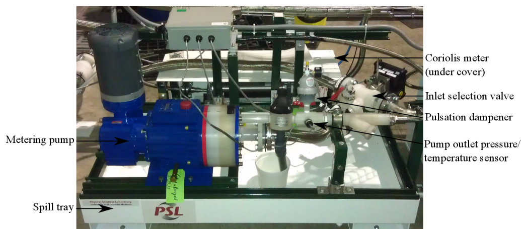
Figure 5. Picture of GdLS pump stand with major components labeled.
