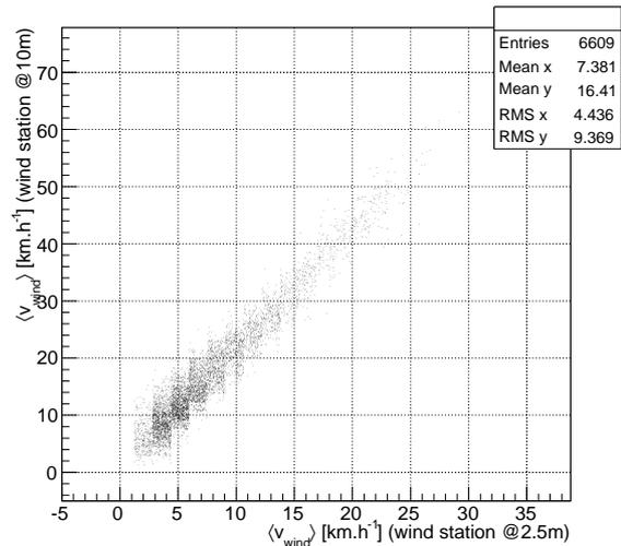
**Fig. 4:** Comparison of wind speeds measurements at CTA-s taken with the anemeter placed at 2.5 m and 10 m above the ground. Courtesy St. Vincent.
