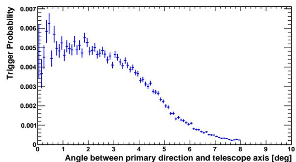
**Figure 1:** Trigger probability for proton showers as a function of the angle between the primary direction and the telescope axis.
