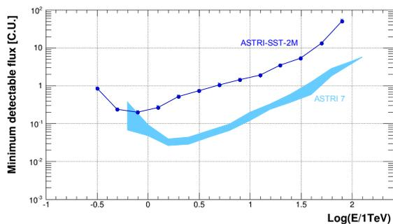
**Figure 4:** The expected differential sensitivity of the ASTRI-SST-2M prototype in Crab Units (C.U.) (blue points). The expected sensitivity of the ASTRI mini-array with 7 telescopes is shown for comparison (blue shaded area) [23].
