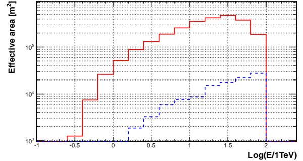
**Figure 2:** Effective area for gammas (red solid line) and effective area for protons times 100 (blue dashed line) after the gamma/hadron discrimination cuts.
